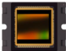
The CMV12000 is a high sensitivity pipelined global shutter CMOS image sensor with a resolution of 4096 x 3072 pixels (super
